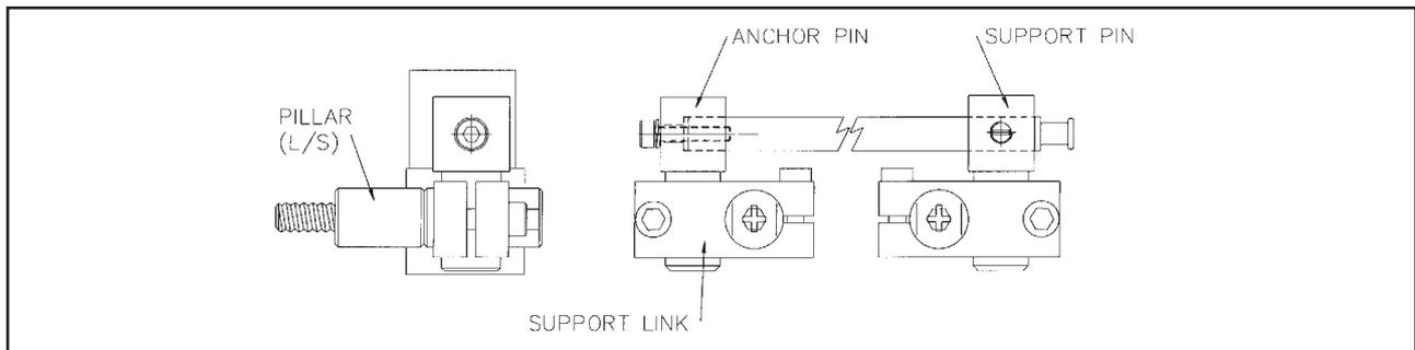
**Figure 5.8 - Microsyn Scale Support Bracket**
