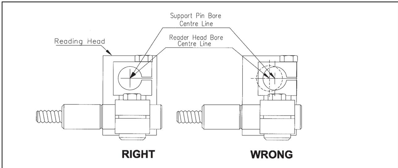
**Figure 5.2 - Reader Head and Bracket Alignment**
