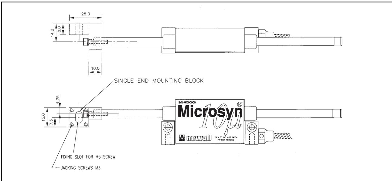
Figure 5.10 - Microsyn Single End Mounting
